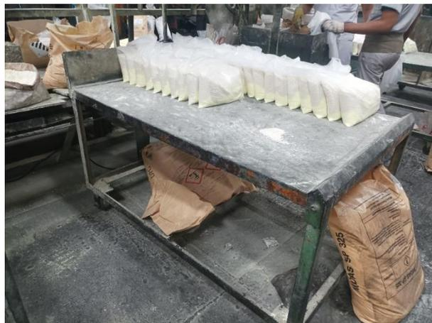
Gambar I.2 Proses Penimbangan Manual (*Chemical Powder*) di PT SRI
