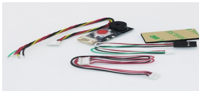
Gambar 1. 7 Safety Switch dan Buzzer
