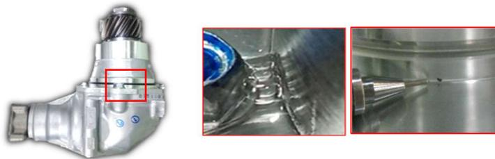
Gambar 1. 2 Bubble Karena Pinhole
