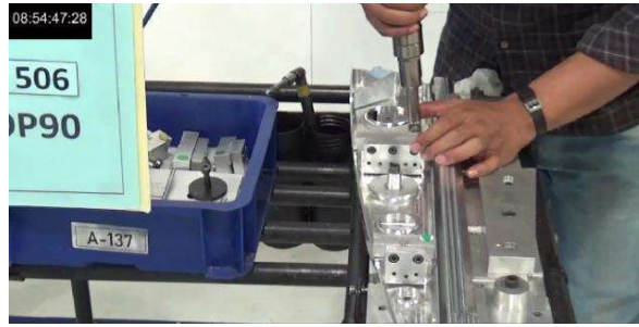
Gambar 1.3 Proses Manual Air Drill
