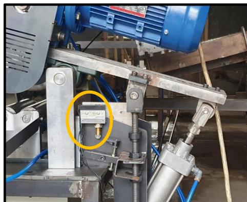
Gambar IV-6 Detail Sensor 5 (*Limit Switch*)
