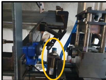
Gambar IV-5 Detail Sensor 1 (*Proximity Inductive*)
