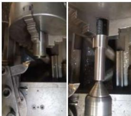
Gambar 2.39 Proses Pembubutan As Housing Bawah
