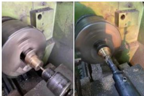
Gambar 2.41 Proses Pembubutan Bronze Bushing 2
