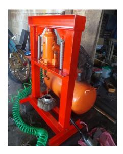
Gambar I.5 Mesin Press Manual 10 Ton
