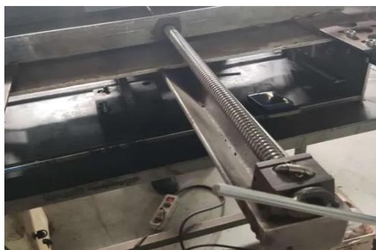
Gambar I. 5. Sistem Pendorong Pada *Pleated Machine*
