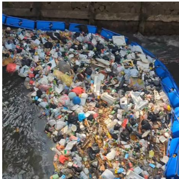
Gambar I.2 Floating trash trapper milik RCI [8]
